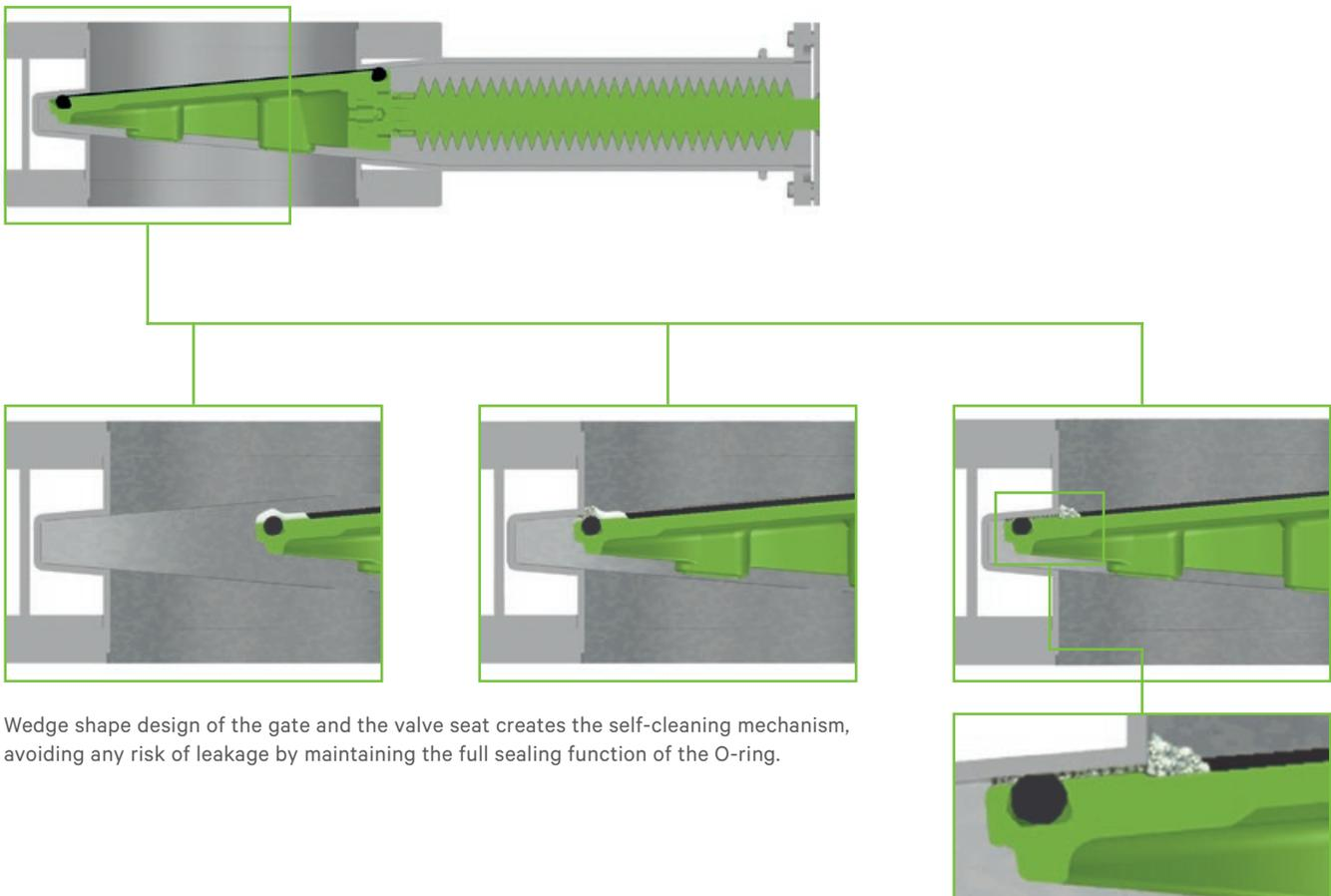
Wedge shape design of the gate and the valve seat creates the self-cleaning mechanism, avoiding any risk of leakage by maintaining the full sealing function of the O-ring.
