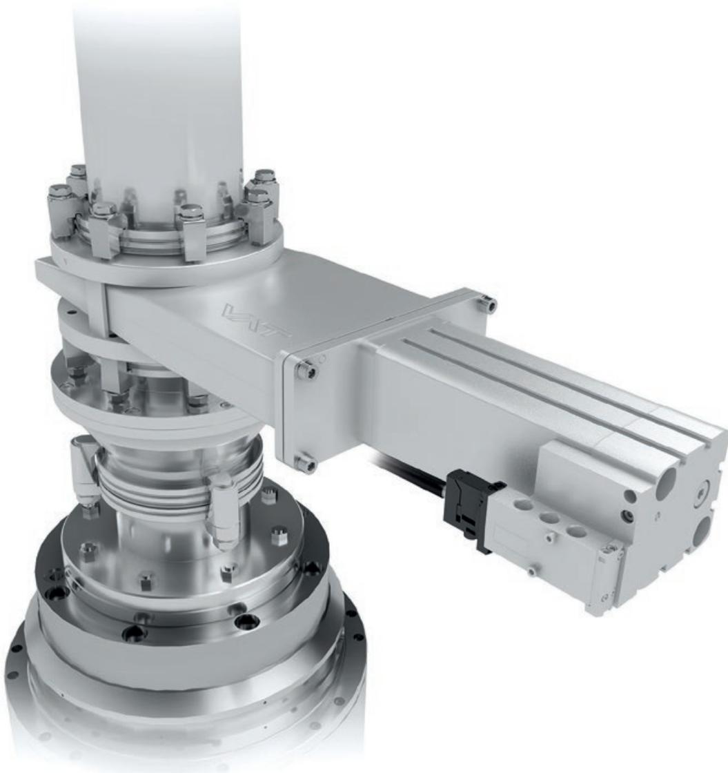
The 09.1 HV gate valve with wedge design is available in manual and pneumatic versions. The standard voltage of the control valve is 24 VDC. For flange connections, customer-specific flanges are possible in addition to ISOKF, ISO-F, CF-F, ASA-LP or JIS. The standard O-ring material is FKM, but other materials are available upon request. In addition, the integration of a soft-pump function is an option as well as providing additional access points for e.g. measuring instruments.
